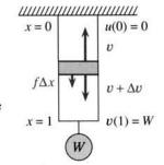
Fig. 7.2 Difference in internal force balances external force
