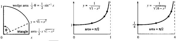
**Fig. 7.5**  $\int \sqrt{1-x^2} \, dx$  is a sum of simpler areas. Infinite graph but finite area.
