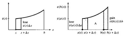
Fig. 5.15 Area from x to b has dg/dx = -v(x). Area v(b)db is added, area v(a)da is lost
