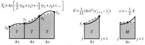
Fig. 5.19 Second-order accuracy: The error prediction is based on  $v = x^2$ .
