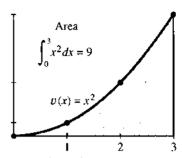
**Fig. 5.6** Rectangles enclosing  $v = x^2$  have area  $(\frac{1}{3}n^3 + \frac{1}{2}n^2 + \frac{1}{6}n)(\Delta x)^3 \approx \frac{1}{3}(n\Delta x)^3 = \frac{1}{3}x^3$ .
