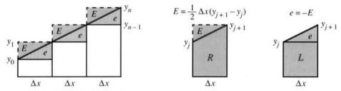
Fig. 5.18 Errors E and e in  $R_n$  and  $L_n$  are the areas of triangles.
