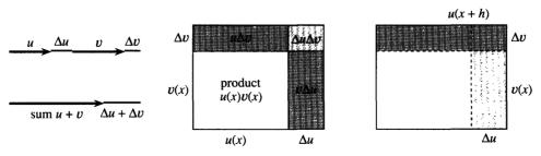
**Fig. 2.13** Change in length =  $\Delta u + \Delta v$ . Change in area =  $u \Delta v + v \Delta u + \Delta u \Delta v$ .
