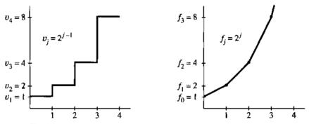
Fig. 1.8 The velocity and distance grow exponentially (powers of 2).
