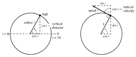
Fig. 1.16 Circular motion with speed I, angle t, height  $\sin t$ , upward velocity  $\cos t$ .
