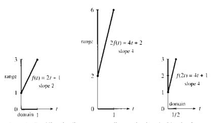
Fig. 1.6 Doubling the distance or speeding up the time doubles the slope.
