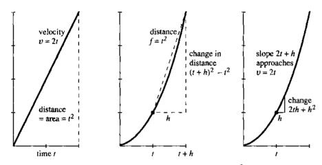
**Fig. 1.12** The velocity v = 2t is linear. The distance  $f = t^2$  is quadratic.
