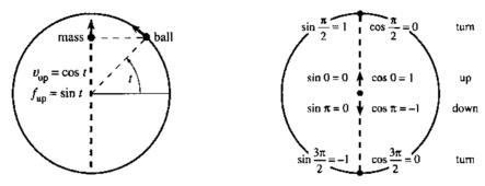
Fig. 1.17 Circular motion of the ball and harmonic motion of the mass (its shadow).
