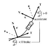
Fig. 12.8 Components of a as car turns corner.
