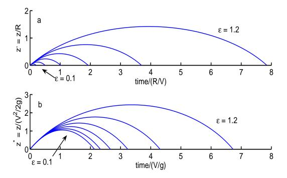
Figure 8: Projectile height computed numerically for several  $\epsilon$  varying from 0.09 to 1.19. The solutions have been nondimensionalized in one of two ways; in (a) using the initial basis set, Eqs. (79) and in (b) using a second basis set built around a zero order solution described in Section 7.3. Notice that for small values of  $\epsilon$  the set of curves in (b) appear to collapse toward one curve, while the set of curves in (a) do not.
