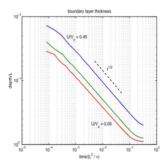
Figure 7: Boundary layer thickness, defined as the depth at which the current was 0.45, 0.15 or 0.05 of the surface value (the three separate curves) diagnosed from the numerical solution of Fig. 6. Note that there was an intermediate (nondimensional) time from about  $5 \times 10^{-3}$  to  $10^{-1}$  during which the boundary layer thickness grew like  $t^{1/2}$ . The similarity solution Eq. (73) holds during this intermediate time and otherwise it does not.
