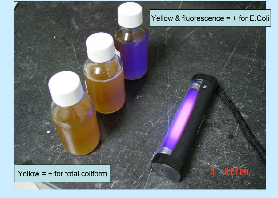
Total Coliform/E.Coli P/A Test showing fluorescence for E.Coli ( = + for E.coli)
