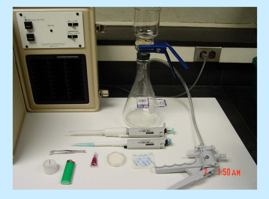
Simplified Membrane Filtration Set-up
