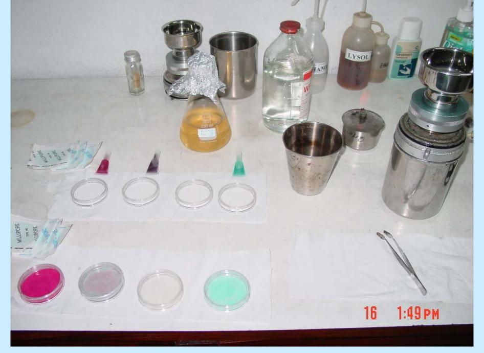
Membrane Filtration Setup with Portable Filtration Unit
