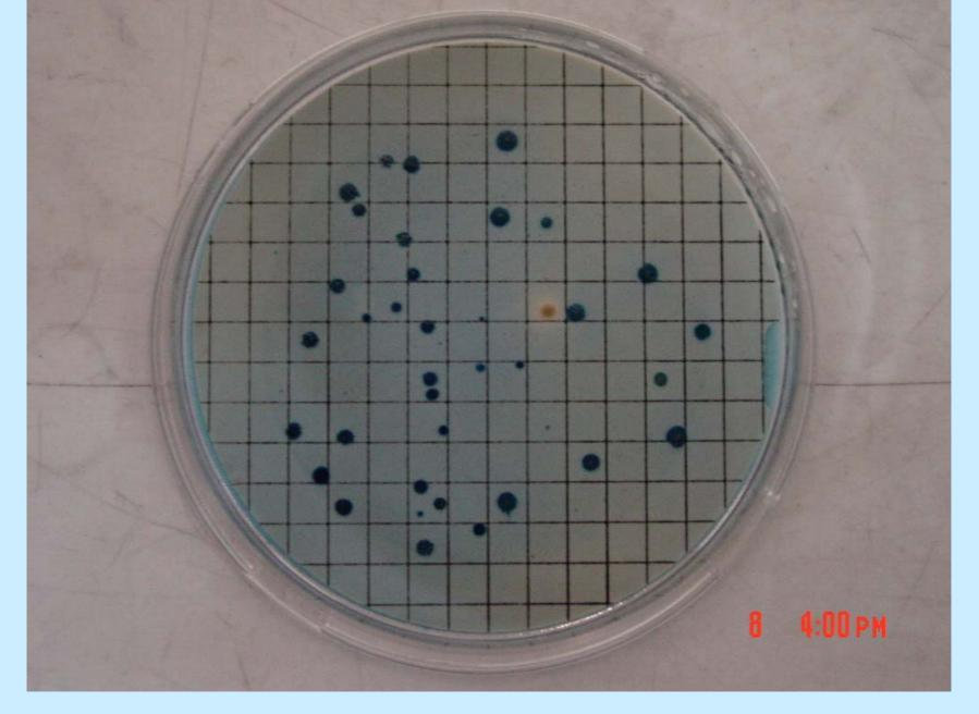
m-FC broth for thermotolerant coliform -> blue colonies after incubation at 44.5 degrees C for 24 hours
