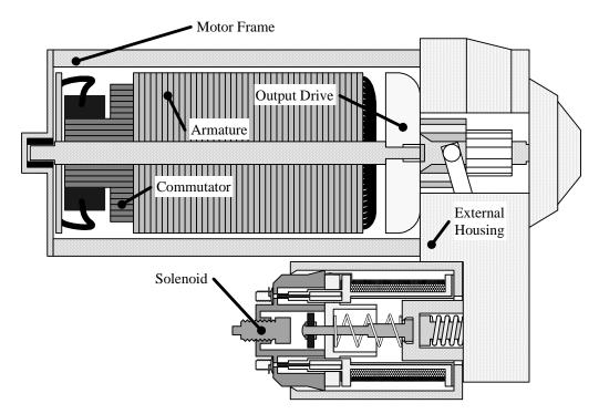
Figure 15: Major Components of an Automotive Starter Motor
