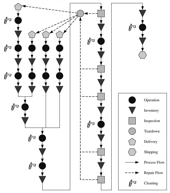
Figure 39: Manufacturing Process Flow For DCS 760
