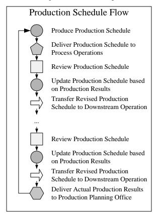
Figure 35: Informational Flows For Coil Production Process
