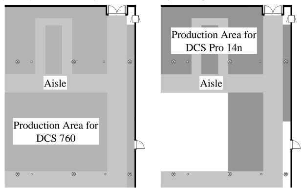
Figure 46: Floor Space Used By DCS 760 Production System
