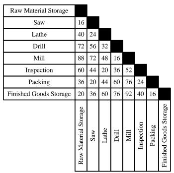
Figure 7: From-To Chart Showing Distances Between Process Elements<sup>68</sup>
