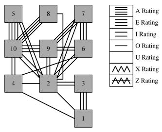
Figure 5: A Sample Physical Flow Relationship Diagram<sup>65</sup>
