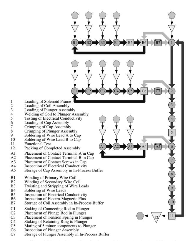
Figure 17: Physical Flow Chart for Automated Production of Solenoid Assembly
