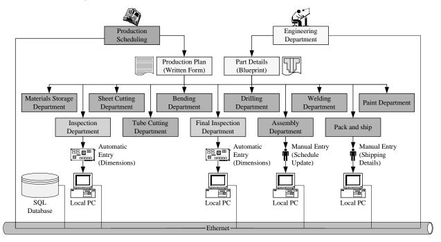
Figure 26: A Sample Informational Flow Block Layout Diagram
