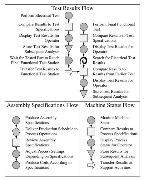
**Figure 34: Informational Flows For Coil Production Process**
