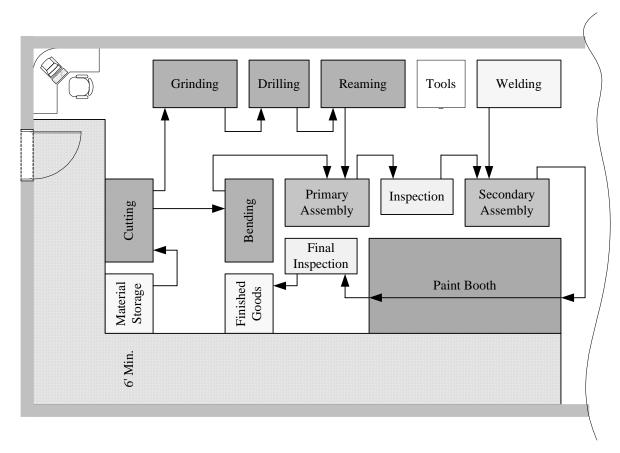
Figure 8: A Sample Block Layout
