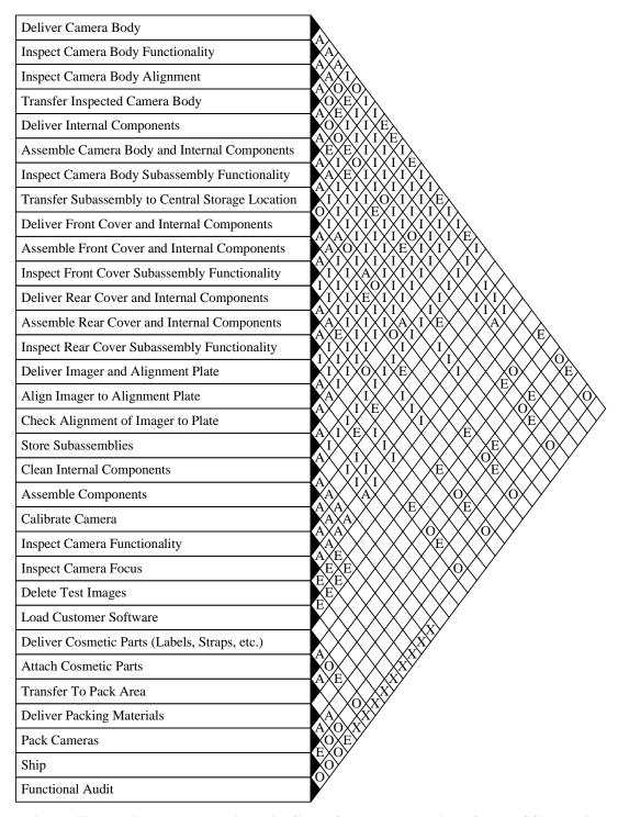
Figure 42: Physical Flow Relationship Chart for the production of the DCS Pro 14n
