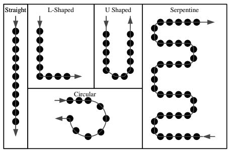
Figure 6: Traditional Flow Patterns Used In Process Layouts<sup>66</sup>
