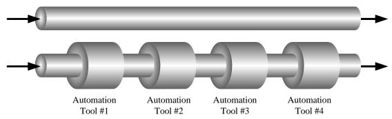
Figure 21: Increasing Local Flow Rates Will Not Increase the Total System's Flow Rate<sup>95</sup>
