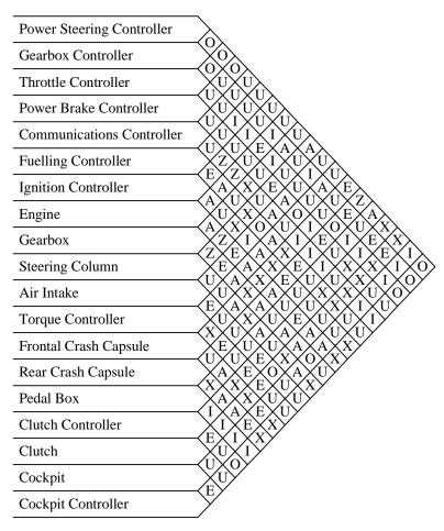
Figure 12: A Physical Flow Relationship Chart For a Formula One Racecar's On-Board Electronics<sup>70</sup>
