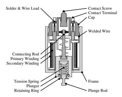
Figure 16: Major components of the Solenoid Assembly
