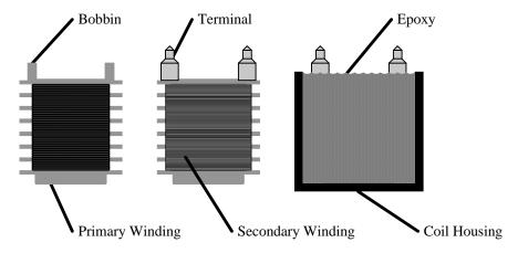
Figure 9: A Representation of the Major Components of an Automotive Ignition Coil
