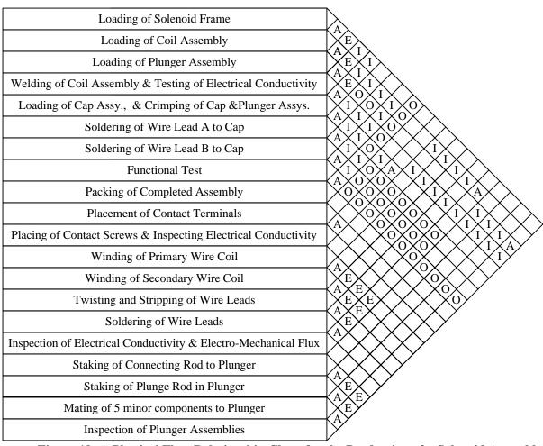
Figure 19: A Physical Flow Relationship Chart for the Production of a Solenoid Assembly<sup>73</sup>
