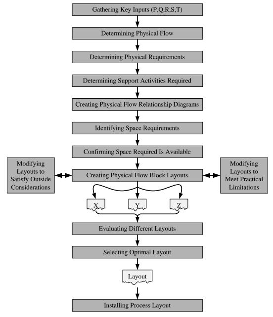
Figure 1: The Systematic Layout Planning (SLP) Process<sup>19</sup>
