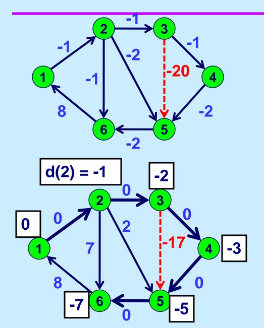
A' = solid lines. They have infinite capacity. The costs are on the arcs.
