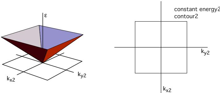
We have studied electrons moving in a box in which the potential energy was zero. Alternatively one could consider electrons moving in a box containing a periodic potential – a simple model for the conduction electrons in a metal with a crystalline lattice. Under these conditions the single particle states can still be indexed by a wavevector  $\vec{k}$ ; however, the energy of each state  $\epsilon(\vec{k})$  need not be quadratic in  $\vec{k}$  nor even isotropic in space.
