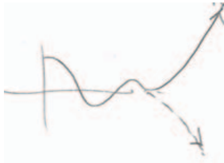
Figure 12: Numerical integration of the Schrödinger equation leads to solutions that diverge up ( \psi \rightarrow \infty ) or down ( \psi \rightarrow -\infty ) beyond some value of x . Bound states are found for values of energies at which the divergence changes from up to down, or from down to up.
