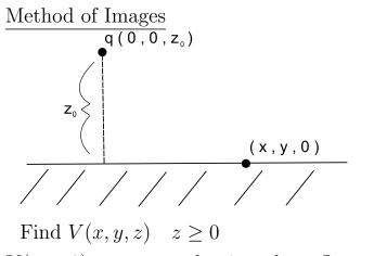
V(x, y, 0) = c on conducting plane, Let c = 0
