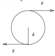
An example is given in the figure, where two forces are applied to a cylinder, attached to a frictionless axis through it center. It is clear that the cylinder will rotate with respect to its axis.
