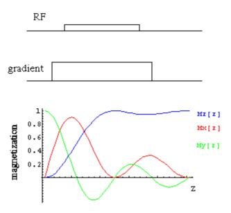
Calculated selective excitation profiles for a weak RF pulse in the presence of a magnetic field gradient. The pulse length is set to rotate the on-resonance spins (at the origin) by 90°, and notice that as the resonance offset increases (with increasing z) the effective rotation angle becomes smaller and most of the magnetization remains along the z-axis. For most images, a shaped RF pulse is employed that creates creates a square magnetization profile.
