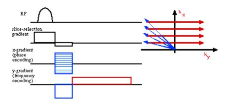
A slice selected 2-D spin warp, gradient echo sequence. Notice that during the phase encoding time the ky vector is offset so that both positive and negative values can be sampled. Since NMR is a coherent spectroscopy, this has the advantage of measuring the phase. The gradient echo in the slice selection direction refocuses evolution of the spins during the selective RF pulse.
