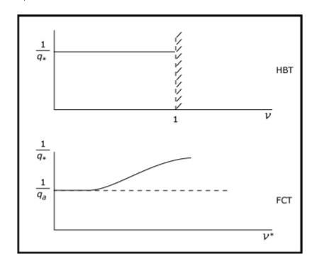
As  $\nu_*$  increases, I increases. This helps to prevent the separatrix from moving onto the plasma surface since less vertical field is required to maintain toroidal force balance.
