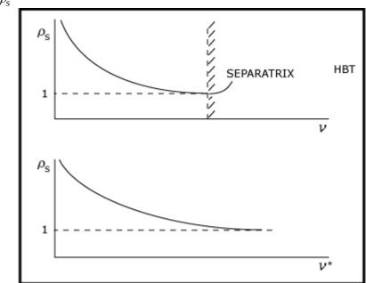
No equilibrium limit. The separatrix does not move onto the plasma surface.
