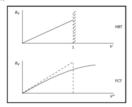
Less vertical field is required. The separatrix stays away from the plasma surface.
