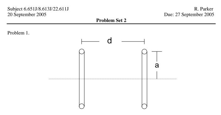
Two circular coils are shown in cross section in the above figure. Each coil has radius **a** and carries a current **I** (in the same direction). The radius **a** is << the separation **d**. A particle with Larmor radius  $\mathbf{r}_L$  and energy **W** is mirror trapped on the axis of the coil system, in the region midway between the coils. The axial extent of the particle's motion is << **d**.
