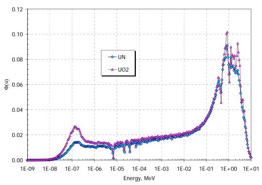
High density of nitride fuel effectively reduces H/HM and thus hardens the neutron spectrum (see above figure). Criticality is also reduced ( $k = 1.2366 \pm 0.0011$ ) due to the lower H/HM and somewhat high neutron absorption by N-14. The reduction in thermal flux component can also be observed from Tables 3 and 4.
