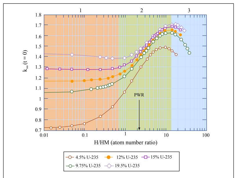
Fig. 1 Initial  $k_{\infty}$  as a function of hydrogen-to-heavy-metal ratio for uranium fueled lattices.
