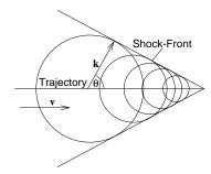
Figure 7.6: Shock-Front arising from coherent addition of waves from all along the particle trajectory.
