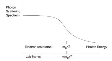
Figure 7.3: Photon scattering spectrum in the lab frame can be thought of approximately as a spectrum flat to  $m_e c^2$  in the electron rest frame, Doppler upshifted to  $\gamma m_e c^2$  in the lab frame.
