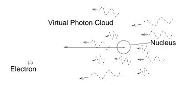
Figure 7.2: In the rest frame of the electron, the electric field of the nucleus is regarded as a "cloud" of virtual photons with a spectrum of energies, which scatter from the electron.
