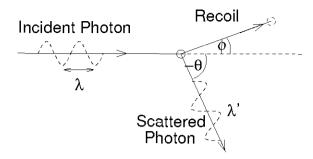
Figure 4.13: Compton scattering geometry in the scattering plane.
