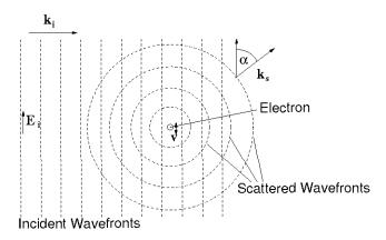
Figure 4.12: Schematic illustration of the process of Thomson Scattering.
