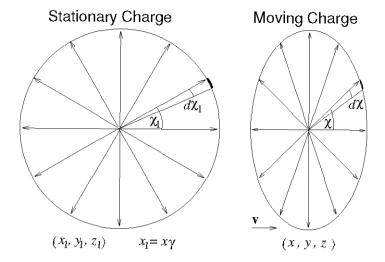
Figure 4.6: Contraction of space which gives the electric field-line distribution of a moving charge.
