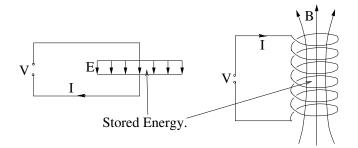
Figure 3.1: Energy obtained from the power supply in "charging up" a capacitor or inductor is stored in the electromagnetic field.
