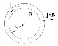
Figure 3.3: Force on a solenoid magnet.
