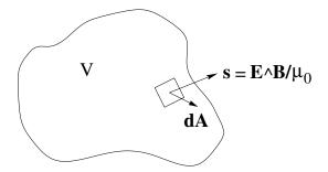
Figure 3.2: Integral of Poynting flux over surface of V.
