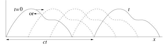
Figure 3.5: Arbitrary solution of the one-dimensional wave equation.
