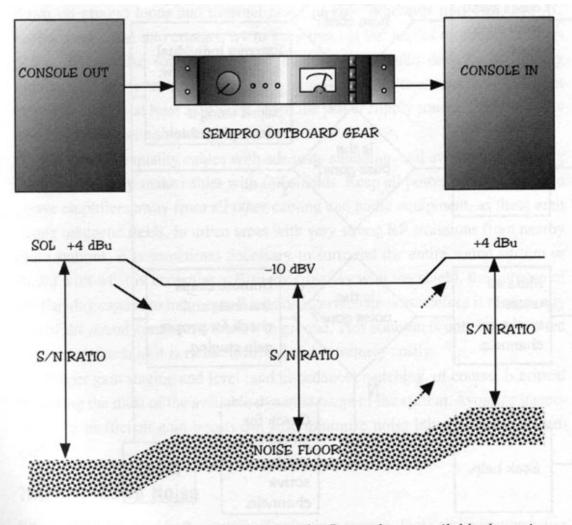
Figure 7.21. Inserting semipro gear into the flow reduces available dynamic range by bringing the noise floor up. Semipro gear not only has a lower SOL (standard operating level) but tends to be inherently noisier as well (higher noise floor).
