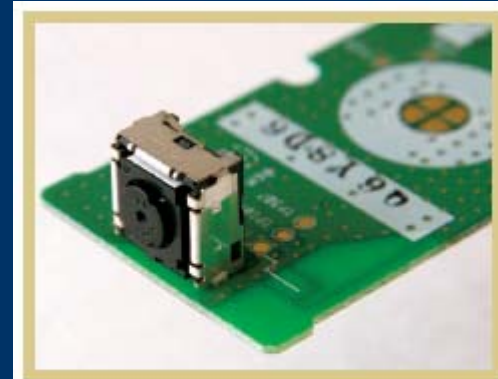
Figure 2. The PixArt IR camera chip. Integrated multiblob tracking minimizes wireless data transmission.
