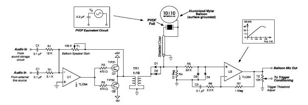
Figure 4: PVDF signal conditioning and interface hardware
