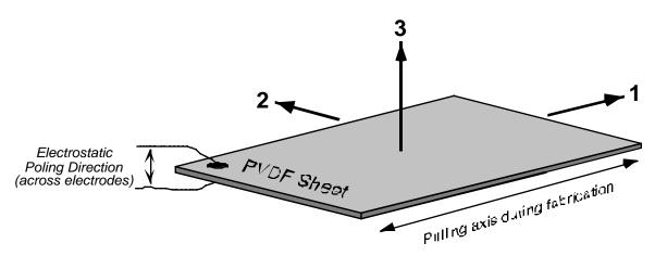
Figure 2: Common definition of PVDF electromechanical axes
