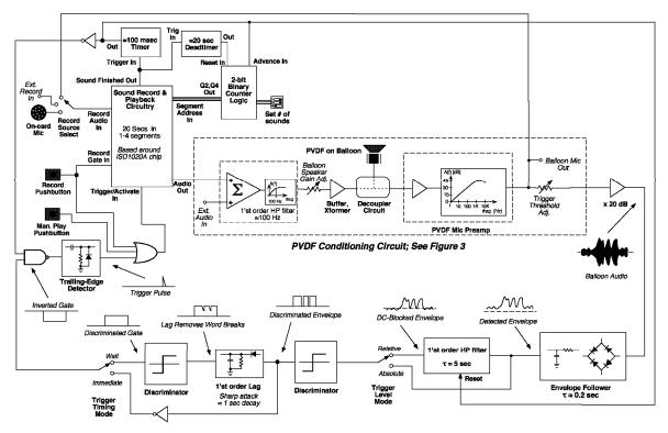
Figure 3: Block diagram of balloon system electronics
