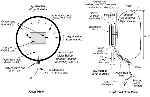
Figure 1: Mechanical structure of balloon-mounted transducer
