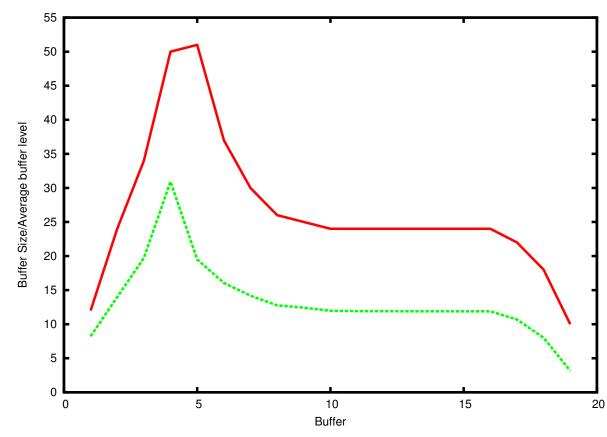
• This shows the ratio of *average inventory* to buffer size with optimal buffers for Case 3.
