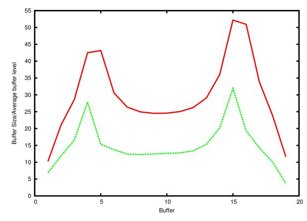
• This shows the ratio of *average inventory* to buffer size with optimal buffers for Case 5.
