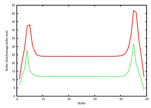
• This shows the ratio of *average inventory* to buffer size with optimal buffers for Case 6.
