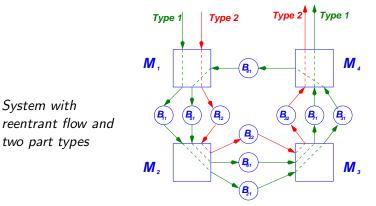
Routes are determined. The number of parts in the loop varies. Semiconductor fabrication is highly reentrant.
