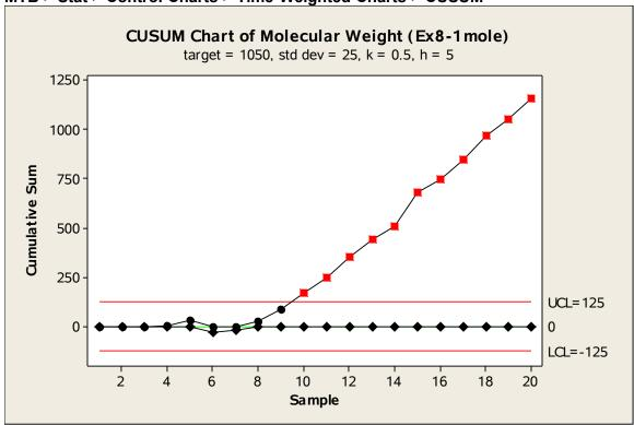
The process signals out of control at observation 10. The point at which the assignable cause occurred can be determined by counting the number of increasing plot points. The assignable cause occurred after observation 10 - 3 = 7.
