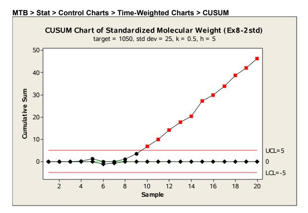
The process signals out of control at observation 10. The assignable cause occurred after observation 10 - 3 = 7.
