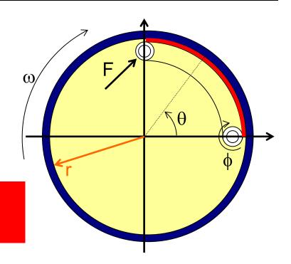
**Then when pad rotates by**  $\Delta \phi$ , **pad:**  $Compression(\theta) = r (\Delta \phi) \sin(\theta)$
