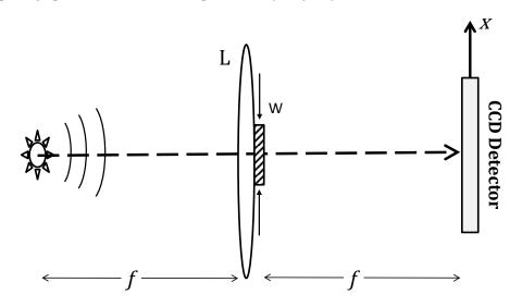
Let's assume the lens is is placed at the plane z = 0 and illuminated by a spherical wave originating on-axis at location z = -f (where f > 0.) Using the paraxial approximation for the spherical wave (y=0),
