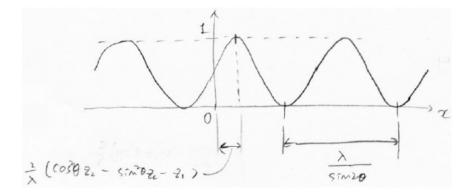
$\therefore$  The period of the fringe is dependent on  $\theta$ . If  $\theta$  increases, the period decreases (finer fringes). Due to the phase shift by  $\frac{2}{\lambda}(\cos^2\theta z_2 - \sin^2\theta z_c - z_1)$ , the whole fringe shifts as  $z_1$  and  $z_2$  change.
