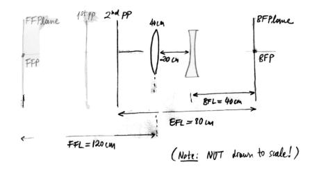
5. An object is placed 200 cm to the left of the first lens of problem 4. Where does the image form and what is the lateral magnification?
