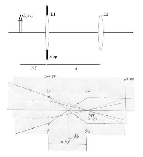
(a) Set the separation distance d such that the Effective Focal Length (EFL) of the combination equals f.
