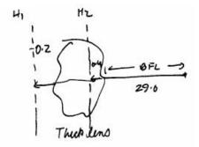
Solution: From the geometry in the figure, we can immediately see that BFL = 29.6 cm and EFL = 29.6 + 0.4 = 30 cm. Just use the principal planes and the imaging condition now.
