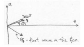
The  $m^{\text{th}}$  plane wave is at an angle  $\theta_m = \theta_0 + m\Delta\theta$
