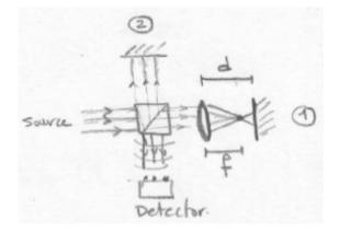
After reflecting off the mirror, the lens is effectively imaging a point source at a distance (d - f) + d = 2d - f; thus it forms a point source image at  $S_i$ , where
