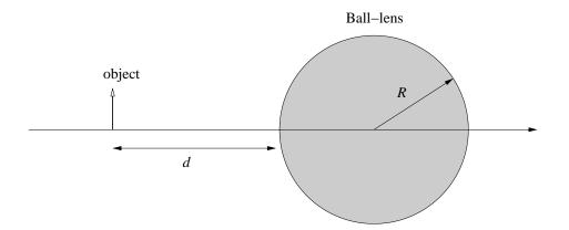
c) An object located at distance d to the left of the back surface of the ball lens, as shown in the schematic, where
