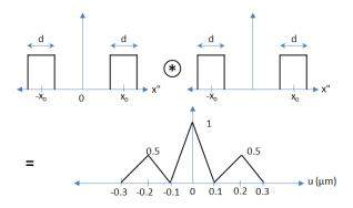
Figure 3: Graphical calculation of OTF.
