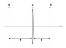
Figure 1: Fourier transforming lens.
