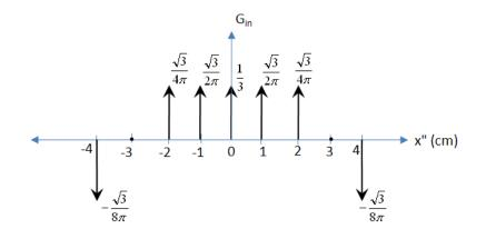
Figure 2: Input signal spectrum.
