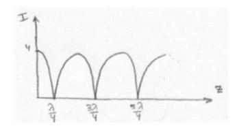
Note that although we did not ignore the time dependence of each wave  $(\omega t)$ , the interference wave is independent of time, thus the term "standing wave."
