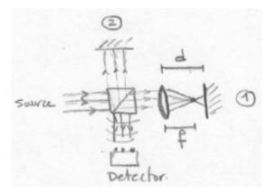
After reflecting off the mirror, the lens is effectively imaging a point source at a distance (d - f) + d = 2d - f; thus it forms a point source image at  $S_i$ , where
