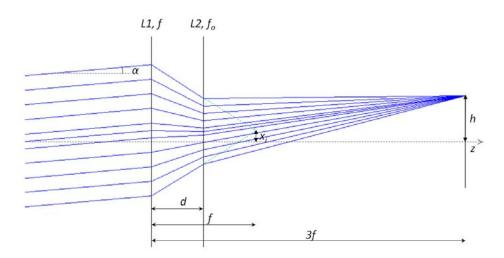
Figure 4: Telephoto lens system.
