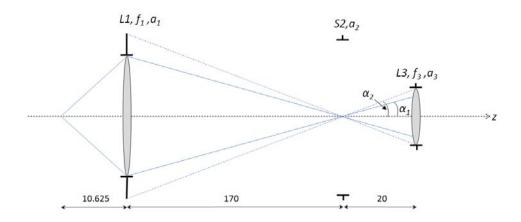
Figure 8: Finding the aperture stop.
