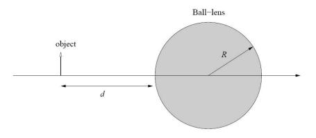
Figure 3: Imaging with a ball lens magnifier.
