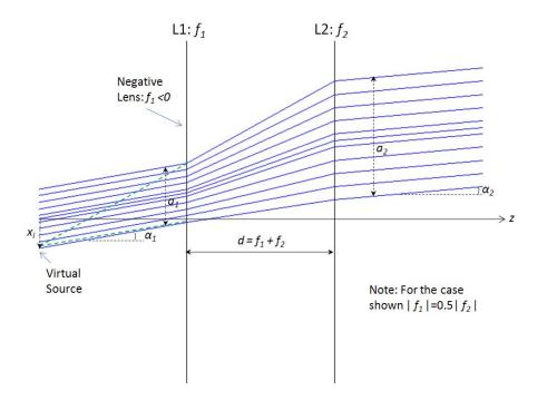
Figure 3: Galilean telescope.
