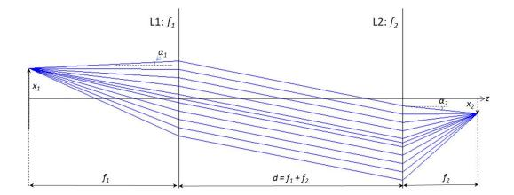
Figure 4: Telescope with finite conjugates.
