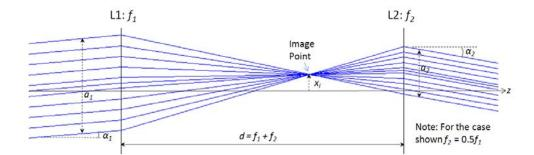
Figure 2: Telescope with infinite conjugates.
