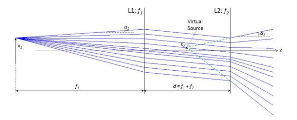
Figure 5: Galilean telescope.
