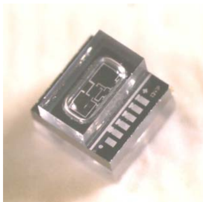
Figure 3.8: Silicon pressure sensor SP15 bonded with glass cover (Courtesy SensoNor AS - An Infineon Technologies Company).
