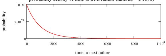
probability density of time to next failure (lambda = 1/1000)
