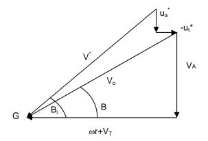
2) (50 pts) A ship captain must purchase a new propeller to replace the damaged one currently installed on his ship. The supplier only has two propellers in stock. Both are fixed pitch, 5 blade Wageningen B-series propeller with an EAR of .45, one has a pitch of 17.1 ft and the other a pitch of 20.9 ft. The details of the ship are as follows:
