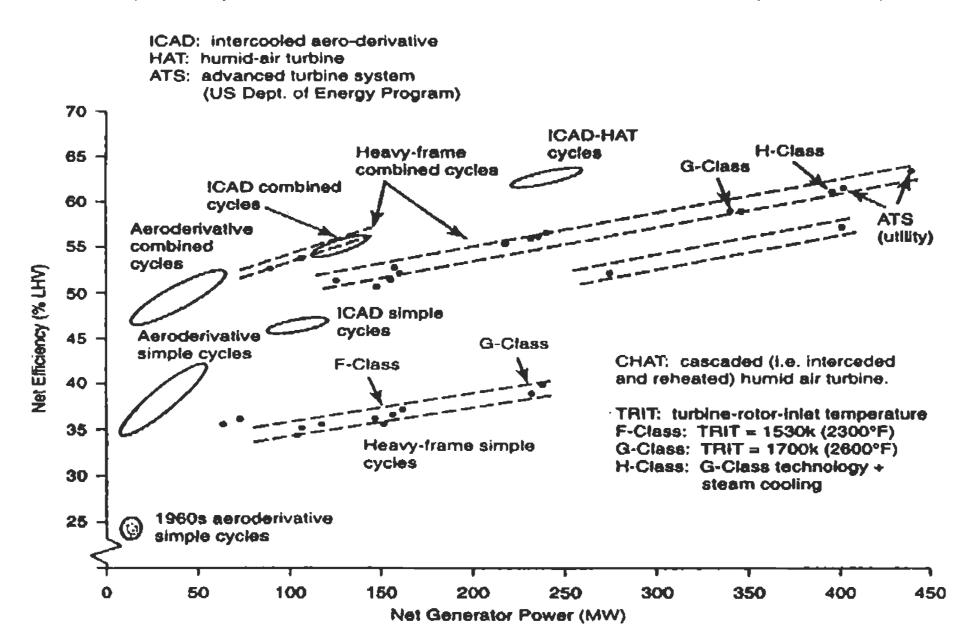
Figure 3. Thermal efficiency versus power of different turbines, and combined cycles (Wilson, and Korakianitis, 1998).
