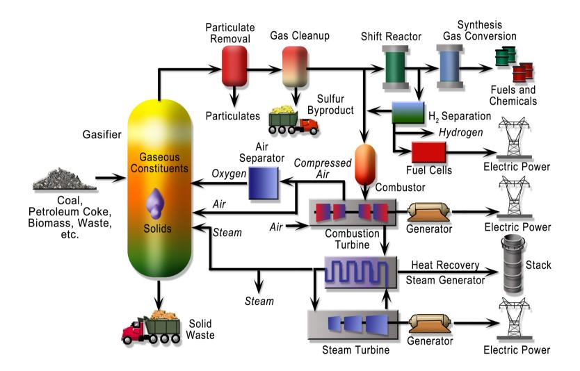
FIGURE 2. GASIFICATION-BASED ENERGY CONVERSION SYSTEM OPTIONS
