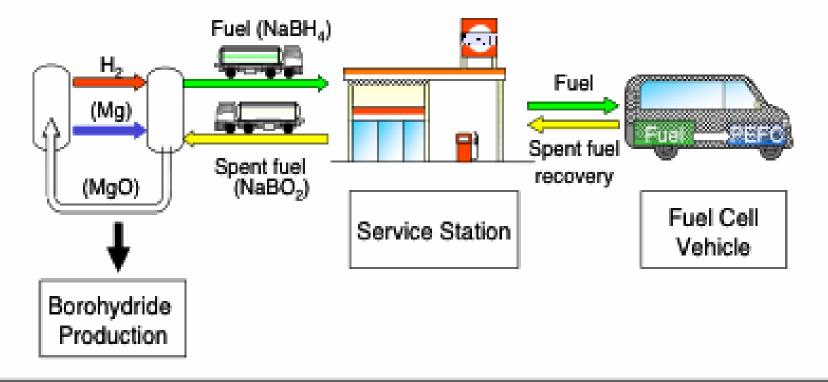
Typical fuel: 30% NaBH4+3%NaHO+67%H2, has 6.6%H2, all by wt. OR <u>66 gH2/L compared to 70 g/L liquid H2 and 23 g/L gas (at 350 bar).</u>
