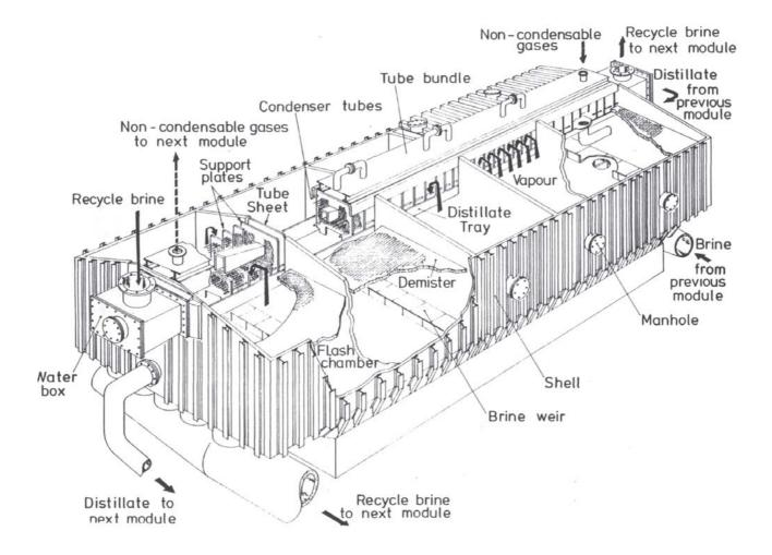
Sectional View of Evaporator Module
