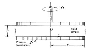
Problem 1: Measuring Viscometric Functions in the Parallel Plate Rheometer [25 points]
