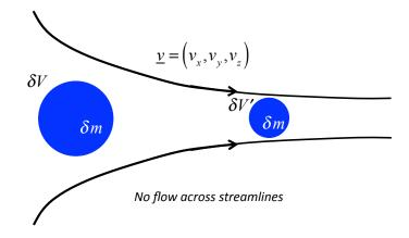
Consider a fluid element with constant mass  $\delta m$  and volume  $\delta V$  moving in a velocity field as shown above. The streamlines are converging and the fluid element may be advected to a new position which has a higher speed. If we assume the most general case, in which the fluid element is compressible, then  $\delta m$  is fixed but  $\delta V$  changes. Note that:
