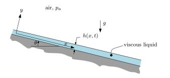
A rigid plane surface is inclined at an angle  $\theta$  relative to the horizontal and wetted by a thin layer of highly viscous liquid which begins to flow down the incline.
