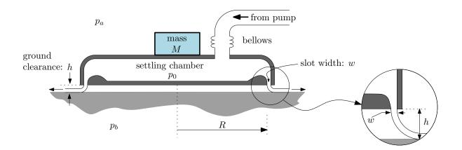
A circular hovering platform of radius R is to support a mass M (its own mass plus a load). A thin, sheet-like jet (width w) is directed downward at the platform's periphery, as shown. The jet is fed from a settling chamber which is maintained at a pressure  $p_0$  by an external pump. The system is to hover at an elevation h which is large compared to the width w of the sheet-like jet, but small compared with R.
