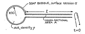
A soap bubble (surface tension  $\sigma$ ) is attached to a narrow glass tube of the dimensions shown. The initial radius of the bubble is  $R_0$ . At t = 0, the end of the tube is abruptly opened.
