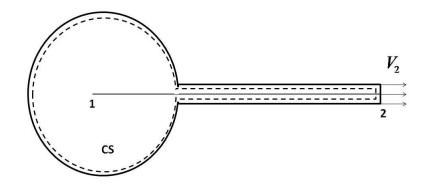
(a) To obtain an expression for R, we will write mass conservation across the moving control volume outlined in the figure above then since the flow is inviscid, incompressible and steady, we can write Bernoulli's equation (conservation of momentum) across a streamline from point 1 to point 2.
