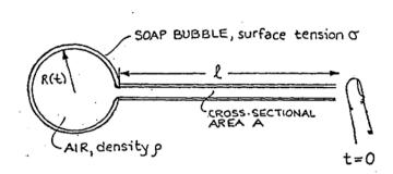
A soap bubble (surface tension  $\sigma$ ) is attached to a narrow glass tube of the dimensions shown. The initial radius of the bubble is  $R_0$ . At t = 0, the end of the tube is abruptly opened.
