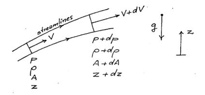
Consider the <u>frictionless</u>, steady flow of a compressible fluid in an infinitesimal stream tube.
