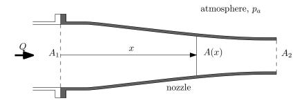
A nozzle with exit area  $A_2$  is mounted at the end of a pipe of area  $A_1$ , as shown. The nozzle converges gradually, and we assum that the flow in it is (i) approximately uniform over any particular station x, (ii) incompressible, and (iii) inviscid. Gravitational effects are, furthermore, taken as negligible. The volume flow rate in the nozzle is given as Q and the ambient pressure is  $p_a$ .
